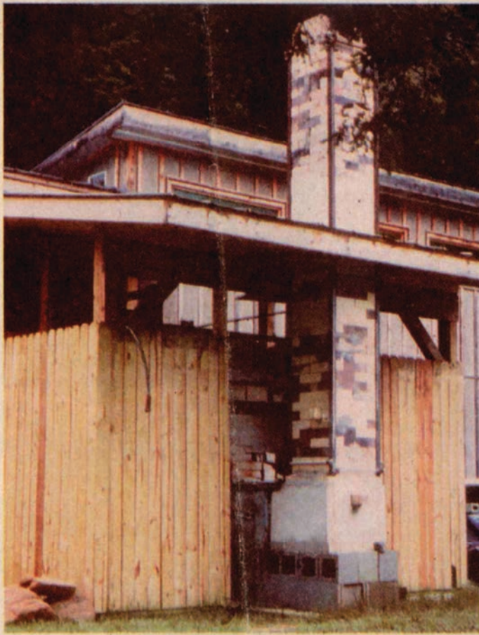
Sue Wasserman photos/SPECIAL TO THE CITIZEN-TIMES Kent McLaughlin's kiln towers over his Bakersville studio. He fuels the furnace with recycled cooking oil from a nearby restaurant.
